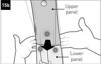
Once top of lower cover has unclipped, the upper cover can then be removed from the lower cover.
