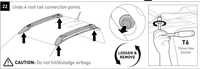
Carefully separate the rail off the vehicle roof, starting from the **REAR**, then moving to the **FRONT** (gradually pry off adhesive tape along the centre of the rail).
